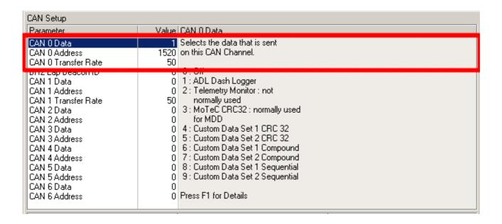
"CAN 0 Data" should be set to 1 (ADL Dash Logger), and the "CAN 0 Address" should be set to 1520 (0x5f0 hexadecimal).
