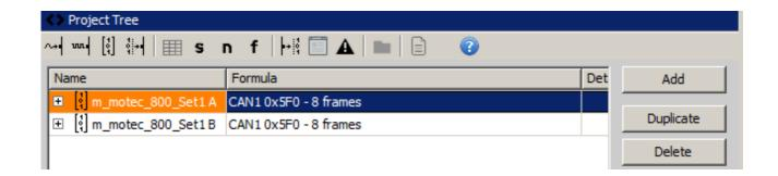
If you open "m\_motec\_800\_Set1A or m\_motec\_800\_Set1B mob", all available CAN inputs should be visible.
