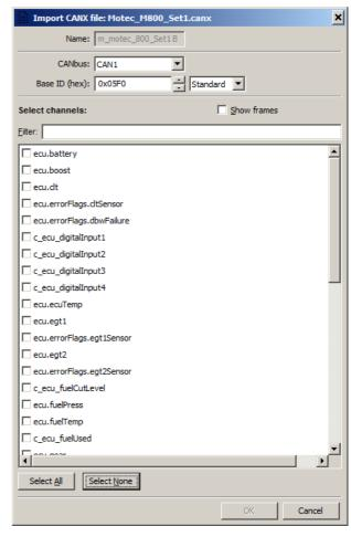
You must select the CAN BUS that will be used for communication (CAN1 or CAN2) and the channels you want to read. In most situations all channels should be loaded (Select All). The project tree should look like the following:
