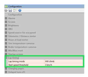
A start of an event is triggered when the vehicle speed ('ecu.speed') exceeds the *Start speed threshold*. The vehicle speed channel ('ecu.speed') is required.
