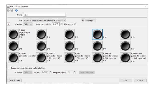
When the driver wishes to adjust a setting, they can press the corresponding button. The rotary encoder will activate, enabling them to change the parameter by turning it.
