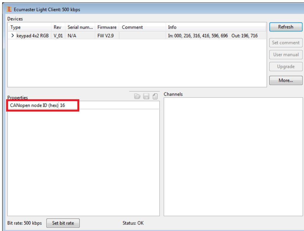
5. [OPTIONAL] If you need to connect these two keyboards to Ecumaster PMU, you need to define *CANopen node ID*=0x16 for the second keypad in the PMU Client software.
