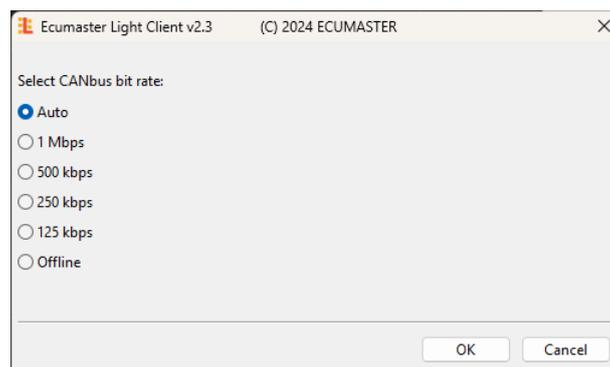
If you use the *Auto* (auto-detection mode) all supported bit rates will be monitored in listen-mode to find the actual bit rate. In the case no frame is received, test frames will be sent to check if any device is able to acknowledge it.
