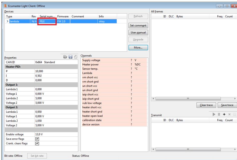
In a similar way to mount a device from ECUMASTER.com server, you are able to mount a device from a local file. It gives you the ability to edit properties and then save it for future use.
