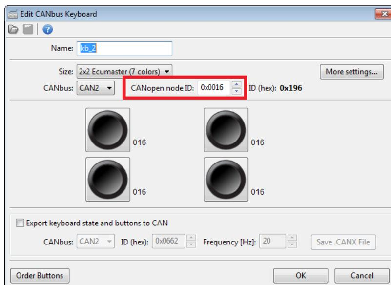
Please do not confuse CANopen node ID with CAN ID. CAN ID describes the address of one frame, while CANopen node ID is a set of frames according to the CANopen standard. And so, for example CANopen node ID = 0x15 the following CAN IDs are used (hex): 0x000, 0x195, 0x215, 0x315, 0x415, 0x595, 0x695, 0x715.
