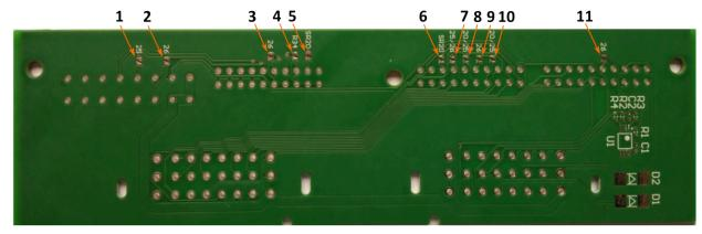
Each jumper consists of two small pads placed next to each other.
