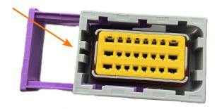
Insert the connector into the adapter socket.
