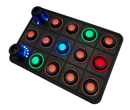
To configure a keyboard, click Add in the Project Tree and then select CANbus Keyboard from the list or click the keyboard icon in the toolbar. Select the 5x3MT from the *Size* menu. The window will look as follows, with encoder positions marked with a frame:
