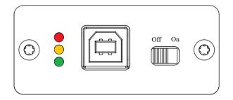
The Ecumaster USBtoCAN is equipped with a 120 Ohm terminator that can be used for CAN bus termination. If you are not using an external terminator, it is necessary to use the one provided by USBtoCAN interface, otherwise the communication will not work. The USBtoCAN terminator can be turned on or off using a switch on the casing.
