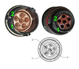
In the **DT** version, there is no internal termination resistor. In the **AS** version, a termination resistor is included, which can be activated by shorting Pin 3 and Pin 4.
