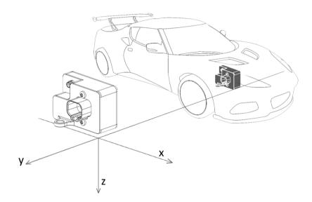
The GPStoCAN V2 module must be mounted with the rubber dampers in a vertical orientation (Z-axis pointing down). Mounting the module to a vertical plane with the dampers oriented horizontally can cause issues with the IMU, as bumps in the road could significantly move the module up and down relative to the vehicle.
