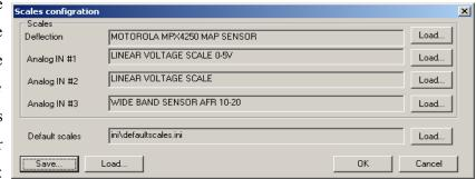
voltage scale, proportional percent scale (for example for TPS), pressure sensors (for example, MPX4250AP, GM 115kPa, Greedy 3Bar), temperature sensors, AFR (narrow band, Zytronix WBO, linear wide band sensor 10-20). The chosen set of scales can be saved in a folder using the option *Save*. It is also possible to load a set of scales, which will be automatically loaded at client start-up.
