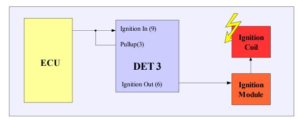
For this signal type, in the menu Setup/Ignition Configuration choose the Ignition Input Type: Hall Effect or optical sensor. As the ignition mode choose the Retard single signal. This mode considers the coil dwell time and copies it in the output signal.
