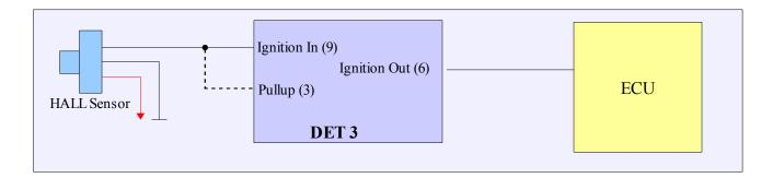
For the Hall's/optical sensors, in the menu Setup/Ignition Configuration chose the Ignition Input Type: Hall Effect or optical sensor.
