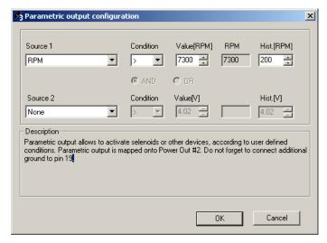
When the engine exceeds 7300 revolutions, the LED diode will turn on. When the RPM drops under 7100, the LED will turn off.
