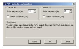
Power outputs can be controlled by PWM within the frequency range of 10Hz-2000Hz. The PWM frequency for every output is defined in the *Setup/PWM Outputs Configuration* window. The *Enable fast PWM (10x)* option increases the output frequency 10 times. PWM controlling is used in all kinds of solenoids ( for example, boost solenoid valve control) or when using an additional injector/ injectors. Values on the PWM table range from 0 - 100%.
