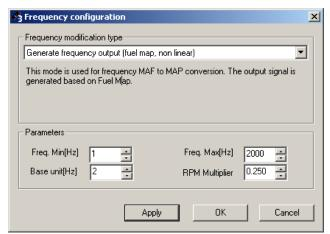
In the frequency MAF sensor to analog MAP sensor conversion, choose the frequency generating mode. The output frequency is generated based on the fuel table values. Frequency of the generated signal is calculated in the non linear way. For this mode, input signal from the *Frequency In* input is ignored.
