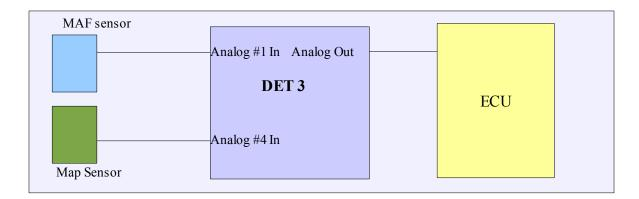
Configuration of the fuel table and analog output at this stage should look as follows:
