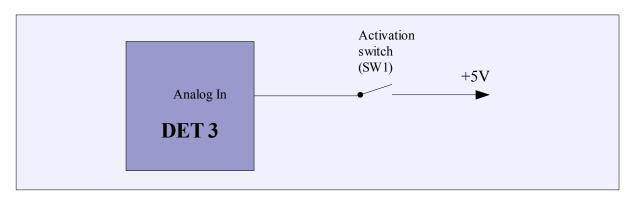
To activate the launch control, apply 5V voltage to a chosen analog input.
