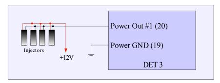
The PWM frequency should be set in range of 30 - 40 Hz. Using the PWM#1 map, it is possible to control output DC (extra fuel dose) from 0% - 100%. A typical example of this usage is a N/A car with a turbocharger. When the boost increases, the DC of additional injectors also increase rising the fuel doses. Due to the additional fuel, the proper AFR can be archived.
