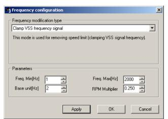
When "clamping" the frequency signal value is necessary (for example, removing road speed governor by limiting frequency of the VSS sensor) it is advised to use "Clamp VSS frequency signal" mode. This mode doesn't require the Fuel Table, so this table can be used for other purposes.
