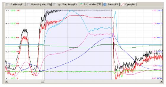
If the input data will be "disturbed" (noisy graph of the rotation speed), the parameter *Filter Power* should be increased.
