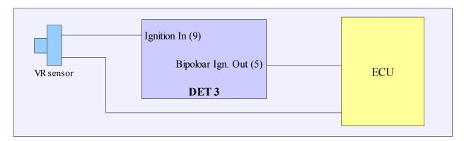
In the case of the balanced signal (differential), VR sensor should be connected to the DET3 device as *single ended*, and connected to the car's ECU as balanced, using both bipolar outputs.
