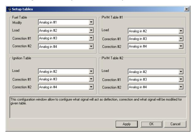
The modified signal for the *Fuel Table* can be chosen among *Analog#1-Analog#4*, *Frequency* and *Zero*. Depending on the kind of a sensor (analog, frequency), a proper input can be chosen. *Zero* means that the value of a modified input signal will be 0. This option is used for the MAF to MAP conversion.
