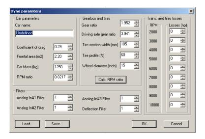
First, RPM ratio factor should be calculated. It is the value which, multiplied by the rotational speed of the engine, will give a current speed of the car:
