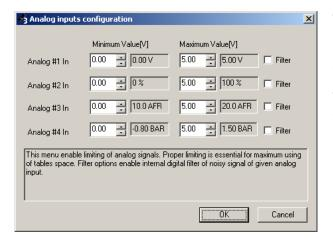
The ranges of the input analog signals can be defined in the Setup/Analog Inputs Configuration window. In this window, it is also possible to precisely define the range of the input voltages and to switch the filtering of the signal using digital low - pass filter. This option can be very useful if the input signal is noisy.
