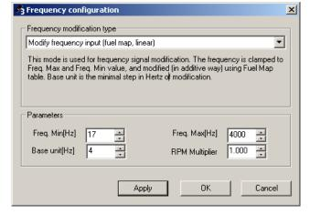
Depending on the frequency range of t sensor, it is possible to use one of two modes of the signal's value change: **linear** or **nonlinear**. For a linear mode, frequency change is linear, proportional to the product of the map's value and the value of the **Base Unit**. Also, value of the output signal is limited in the range defined by the **Freq. Min and Freq.Max**. units. This mode is used for sensors with frequency range not higher than 500Hz.
