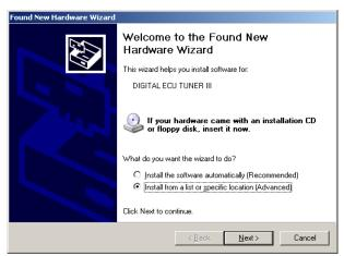
The above directions should be repeated for every new equipment found by the computer. If FTDI drivers of FTDI brand are already installed on a computer, the information about finding a new equipment will not appear and the drivers' installation will not be necessary. After a successful installation, a client can be started.
