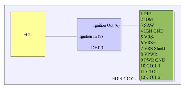
For this type of signal, in the menu Setup/Ignition Configuration choose Ignition Input Type: Hall Effect or optical sensor.
