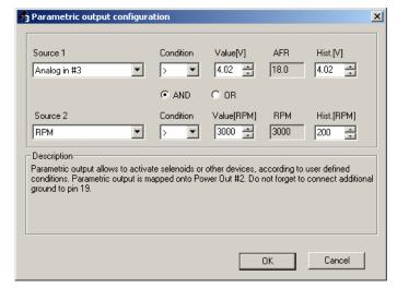
In Analog In #1, there is connected the TPS sensor. The NOS system will be activated if the throttle body is fully open (TPS voltage over 4.0V) and RPM are higher than 3000.
