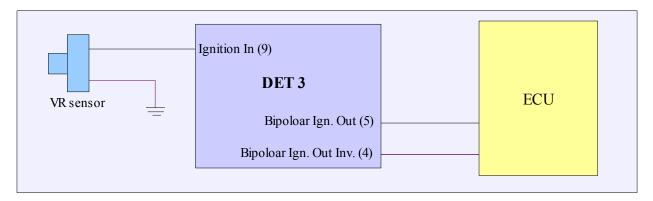
Polarity of the sensor is crucial in case of the balanced signal. Reversed connecting will cause an inability to start the engine or errors in controlling the ignition.
