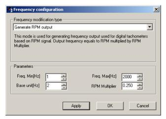
It is possible to generate frequency signal for digital tachometers (where signal is received from ECU and not from the ignition coil.) Frequency of the output signal depends on the current engine speed mulitplied by the *RPM Multiplier* factor, which is used for adjusting the signal to a specific tachometer.
