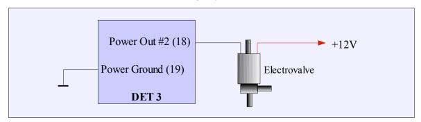
The diagram below describes a way of connecting the 3 way electrovalve used to control boost for the turbocharger with the integrated wastegate.
