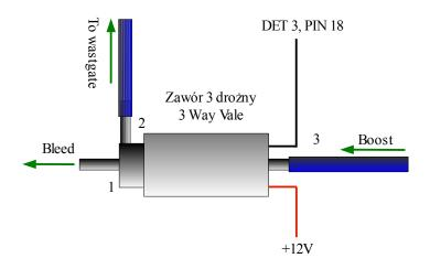
The described valve is opened between the endings 2-3, if it's not powered. With the power on, the opened connection is between 1-2 endings.
