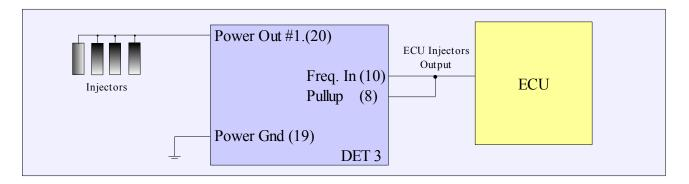
To activate the option of the direct controlling of the injection time, choose *Setup/Injection Control Configuration* from the options, then choose *Injection control type: Full group input, Power Output #1*.
