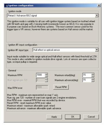
**Ignition Mode** – choosing the ignition mode, suitable for the ignition system of the modified vehicle
