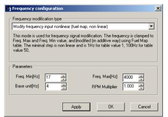
In the **nonlinear** mode, table values are rising in the exponential way. There is a comparison of the frequency change value for the linear and nonlinear mode on the chart below:
