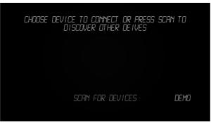
After several seconds a list of found Bluetooth devices will appear. Choose EMUBT device. If EMUBT device will not appear on the list, check connection between EMU ECU and Bluetooth module and LED status.
