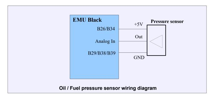
Common pressure sensor pin-out
