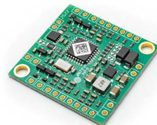
CAN Switch Board
